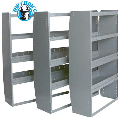
**HD-SWP Series Adjustable Shelving** Contains a 12" deep top tray with a 2" lip, one 14" deep shelf with a 2" lip, and two 14" deep shelves with a 4" lip. Contoured end panels provide flush fit to van side to maximize aisle space. Shelf gussets and a full floor rail provide extra strength. Available in three widths:
